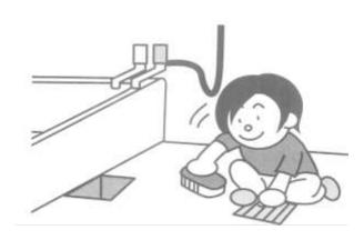
The flow of drain water will become worse if hair and other filth is allowed to clog the drain. Remove the eye-plate and unpleasant-smell trap, and frequently clean them after use.
